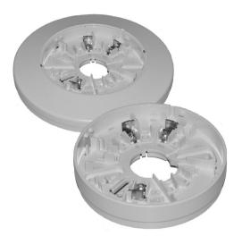
The FAA-440 Analog Bases come in two sizes (4 in. [10 cm] and 6 in. [16 cm]) and two models (Standard and ISO which has a built-in isolator). They are used in combination with FAP-440 and FAH-440 analog addressable detectors to provide early fire warning for life safety and property protection.
